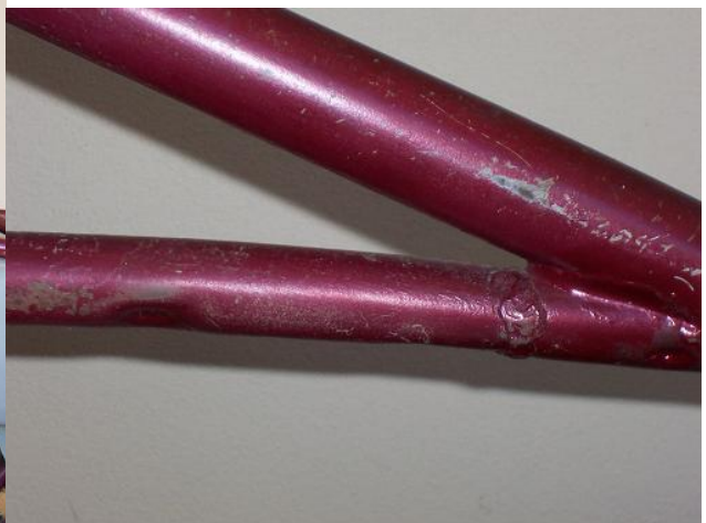
Pictures showing slight kink and small dent in frame
