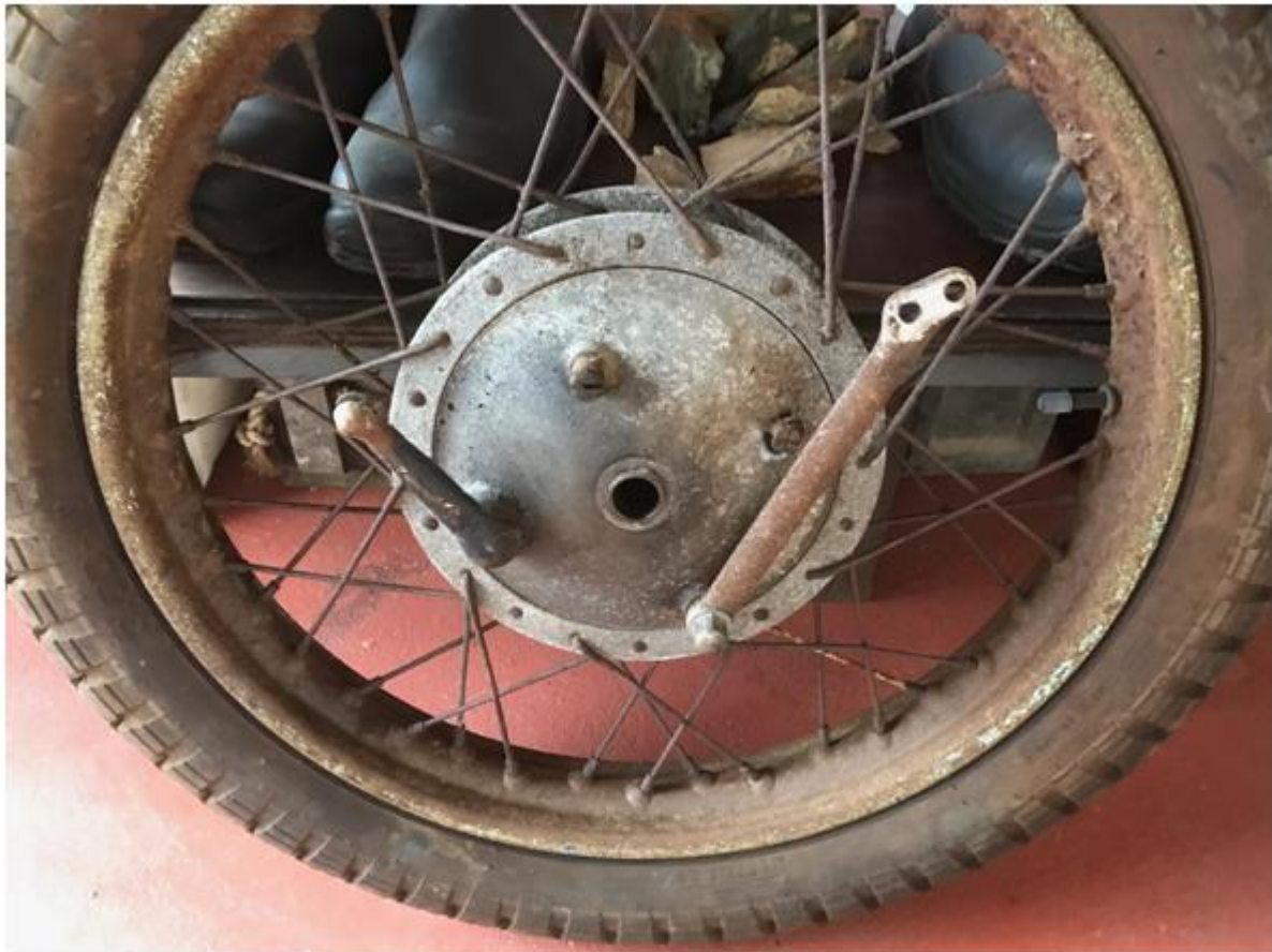
19" Front Wheel (full-width hub)
